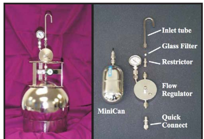
Figure 1 - CS1200E and 6L Silonite Canister (left). Flow controller components disassembled (right).
