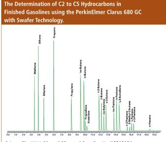
Column: Elite-WAX, 30 m x 0.25 mm x 0.5 µm Part No. N9316404 and Al<sub>2</sub>O<sub>3</sub> PLOT/Na<sub>2</sub>SO<sub>4</sub> 50 m x 0.32 mm Part No. **N6107777**
