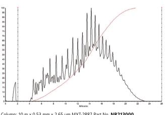
Column: 10 m x 0.53 mm x 2.65 µm MXT-2887 Part No. NR213000
