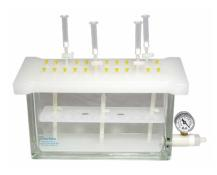
the stationary phase, metered by the stopcocks, to control the speed of the extraction process and the sample flow. Waste and wash solvents are discarded and analytes are collected in sample tubes below the manifold completing the extraction. For your convenience, manifold kits are supplied in either 12 position or 24 position configurations.
