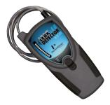
minute leaks of any gas with thermal conductivity different from air. The reference gas inlet draws in ambient air for comparison to air drawn into the sample probe. A leak is detected by both LED bar graph display and audible alarm.
