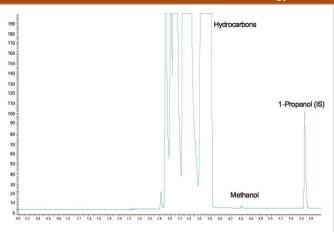
Column: Elite-1 30 m x 0.53 mm x 5.0 µm Part No. **N9316052**
