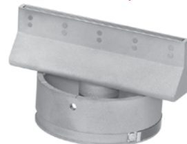
Three-slot Air-acetylene 10 cm
