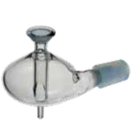
Baffled Cyclonic Spray Chamber Part No. N0791352
